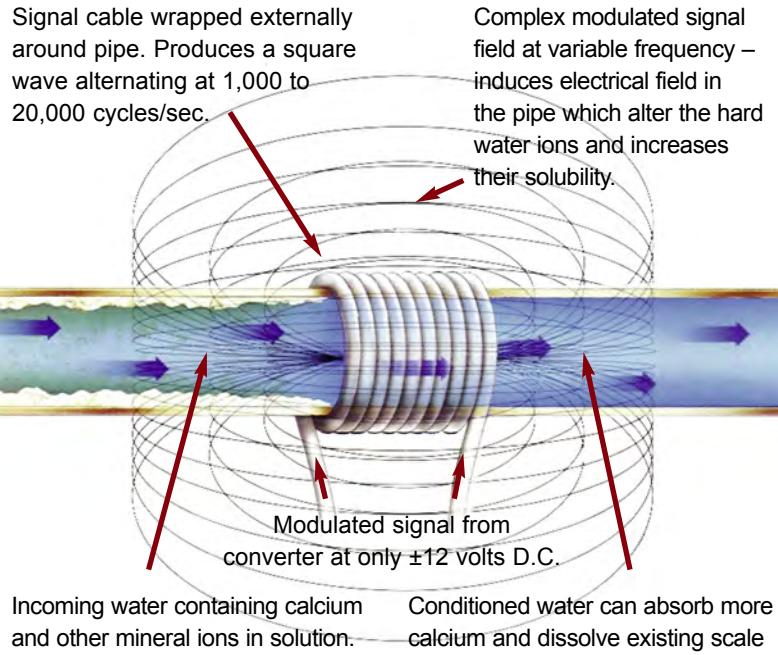
**Patented Technology. Used successfully for over 10 years to de-scale water systems**
